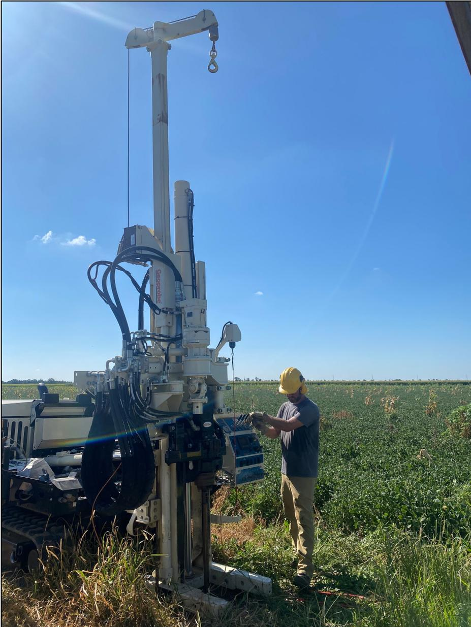
Electrical conductivity (EC) logging provides lithologic information about soil conductivity and resistivity
