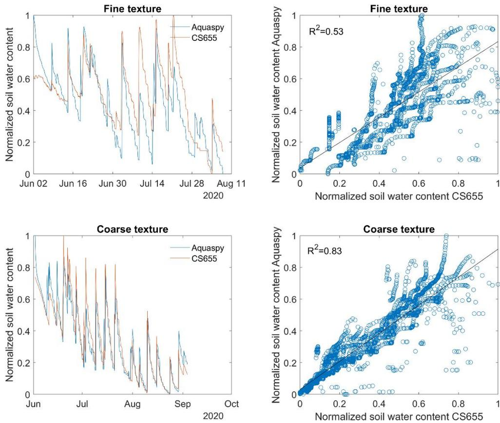
**Figure 2.** Profile (0 to 28 inches) soil water storage determined using the capacitance probe (red line) and an array of four calibrated CS655 soil water reflectometers (black line). Profile soil moisture of sensors located in the A) fine texture (Silty clay loam) soil and B) coarse texture (Loam, 46% Sand) soil. Dash horizontal lines represents the average profile soil moisture for each sensor over the entire time series.
