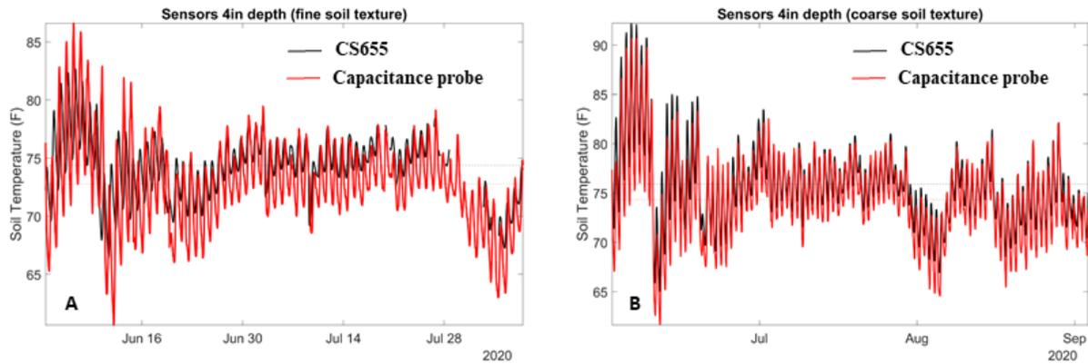
**Figure 2.** Surface soil temperature at 4-inch depth determined using the AquaSpy probe (red line) and an array of four calibrated CS655 soil water reflectometers (black line). Soil temperature from the sensors located in the A) fine texture soil and B) coarse texture soil. Dash horizontal lines represents the average profile soil moisture for each sensor over the entire time series.
