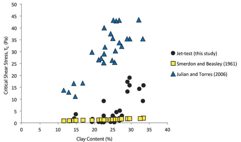
Figure 19. Comparison of jet-test results and estimates of critical shear stress from empirical equations. Note that although Julian and Torres (2006) use percent silt-clay data points are plotted based on percent clay in order to facilitate comparison.
