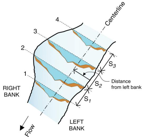
Figure 4. Plan view of transect layout and spacing for use in stream and sediment volume calculations. Distances between transects (e.g.,  $S_1$ ,  $S_2$ ,  $S_3$ ) are measured along the established centerline of the stream. Volumes are calculated by multiplying the cross-sectional area of each transect by the spacing to the next transect.
