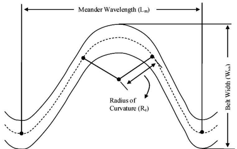
Figure 5. Meander geometry measurements.
