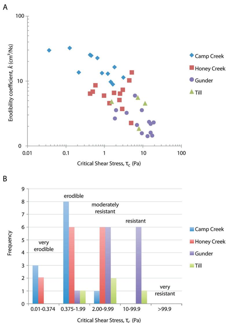
Figure 17. A) Relationship between critical shear stress and the erodibility coefficient ( $k$ ) by stratigraphic member; B) Frequency distribution of critical shear stress values from jet-test results by stratigraphic member.
