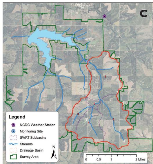
Figure 2. Surveyed and delineated areas of (a) Banner Creek Lake Watershed, (b) Centralia City Lake Watershed, and (c) Atchison County Lake Watershed. The surveyed area (Devlin and Boyer, 2012) is outlined by the green line, while the drainage basin for the USGS gage station is outlined by the red line. The stream network and subwatershed boundaries are respectively colored with blue and orange.
