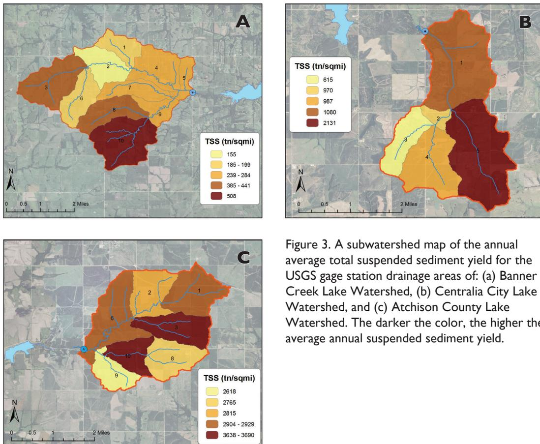
Figure 3. A subwatershed map of the annual average total suspended sediment yield for the USGS gage station drainage areas of: (a) Banner Creek Lake Watershed, (b) Centralia City Lake Watershed, and (c) Atchison County Lake Watershed. The darker the color, the higher the average annual suspended sediment yield.
