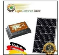
I encourage producers to use the power output portion of the charge controller to power the pumps (rather than hooking direct to the battery). The advantage is that the charge controller will stop the pump if the battery gets below 10.5 volts. Draining batteries at lower voltages can damage the battery. Connecting to a battery directly can run the battery flat if a water line were to break or a tank overflow for some reason.
