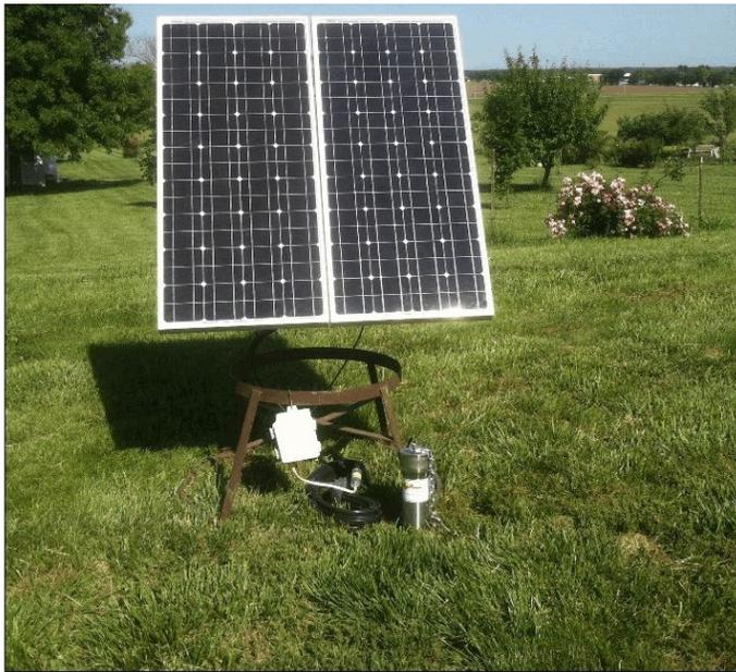
**Figure 1.** Solar pump demonstration unit.
