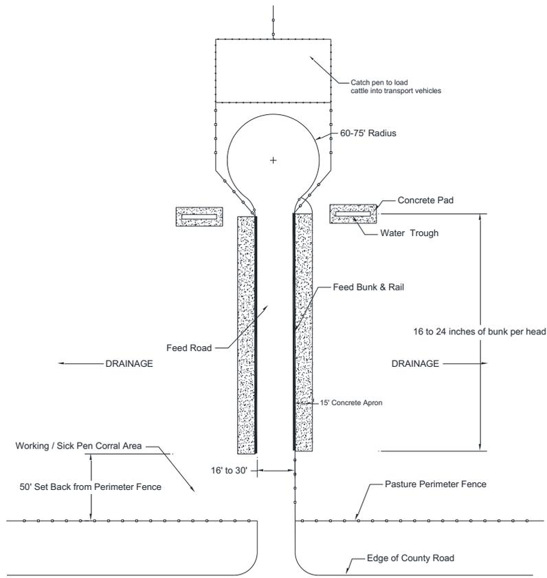
**Figure 2.** Design showing bunks on both sides of a road to feed either one or two pastures.
