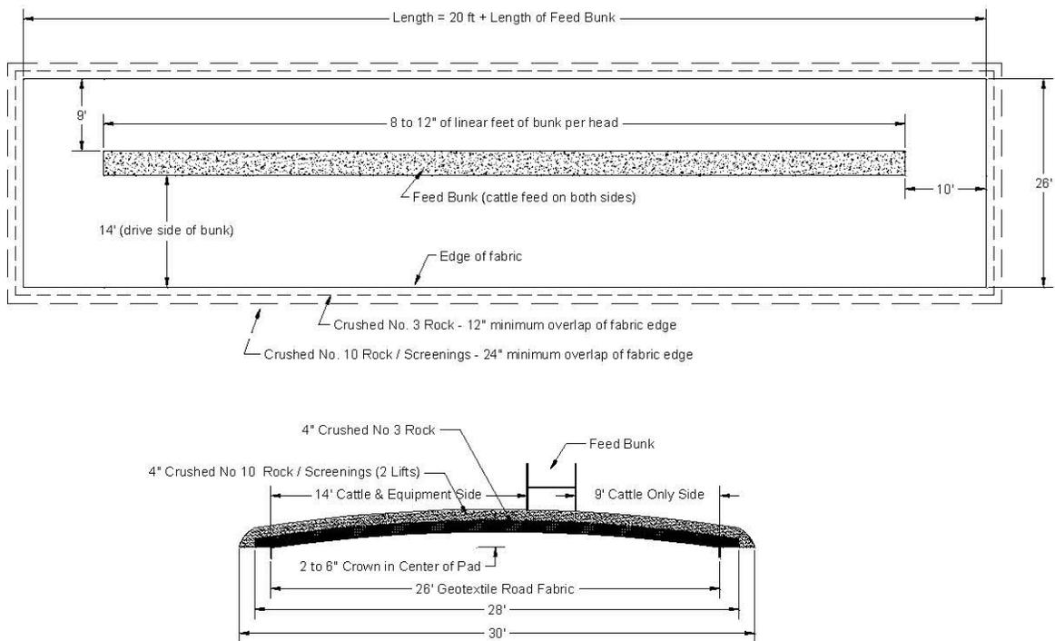
**Figure 1.** Diagram, including example measurements, of permanent feed bunk pads.
