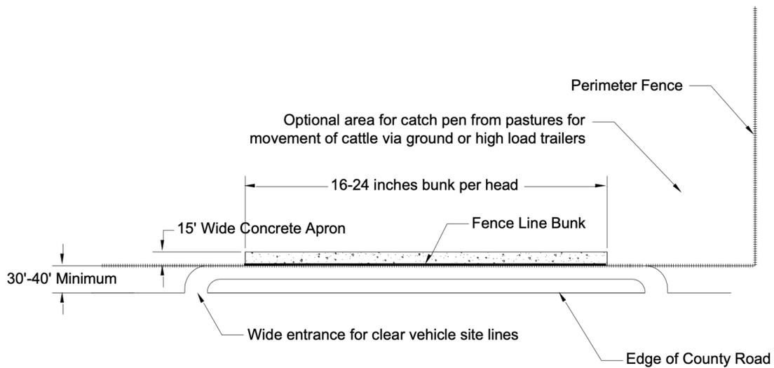
**Figure 4.** Example of a fenceline feed bunk located along the edge of a pasture or cropping field.
