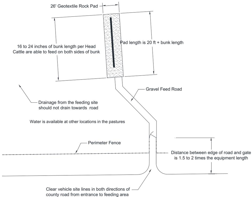
**Figure 3.** Example of a pasture feeding site that is moved away from access road along a ridge to maximize infiltration between the feeding site and road drainage channels.
